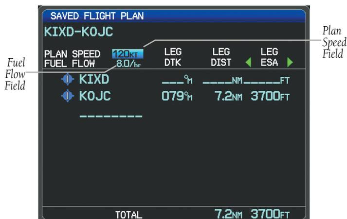
Plan Speed and Fuel Flow (Saved Flight Plan Page)
