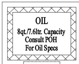
On Exterior of Gascolator Door (Underside of Fuselage)
