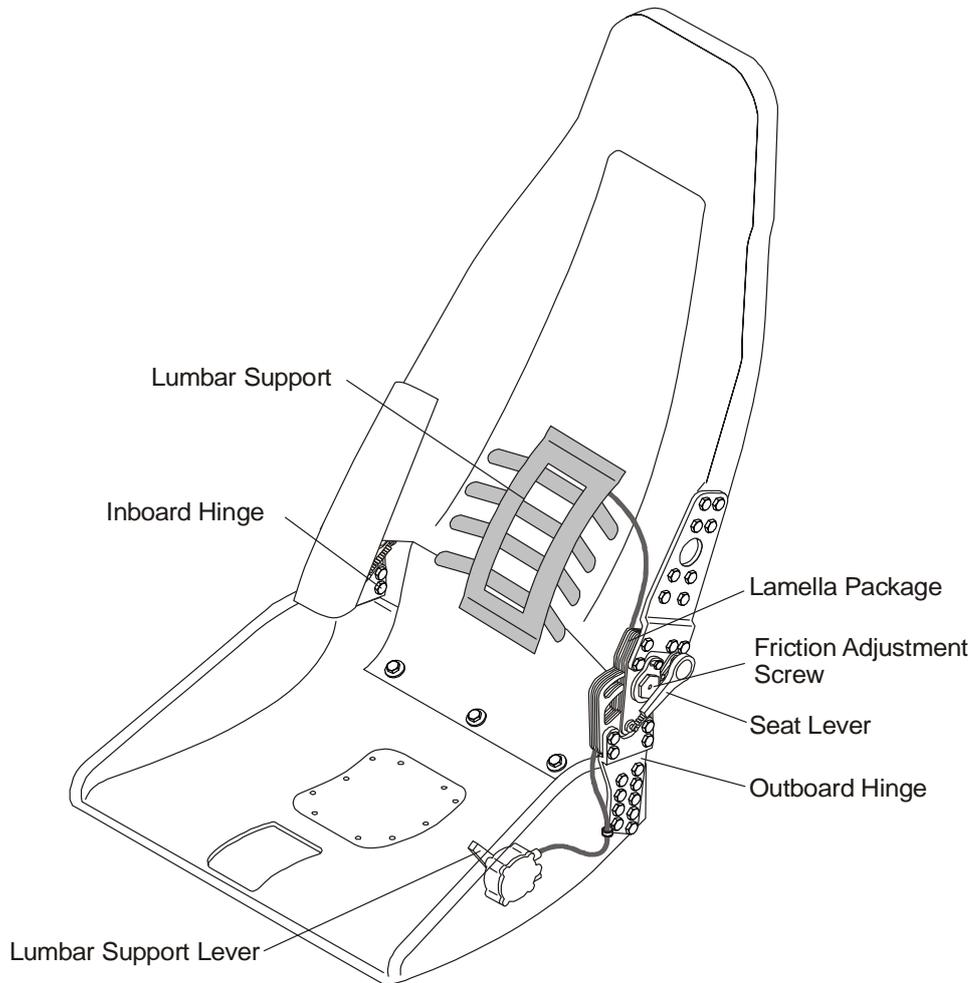
*If seats with adjustable backrest are installed (OÄM 42-259):*
