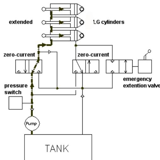
The operating mode for the retraction of the landing gear is shown in the next Figure. While energizing the right hydraulic valve, the fluid flow in the hydraulic system is started due to different piston areas of the landing gear cylinders although the pressure on both sides of the system is equal.
