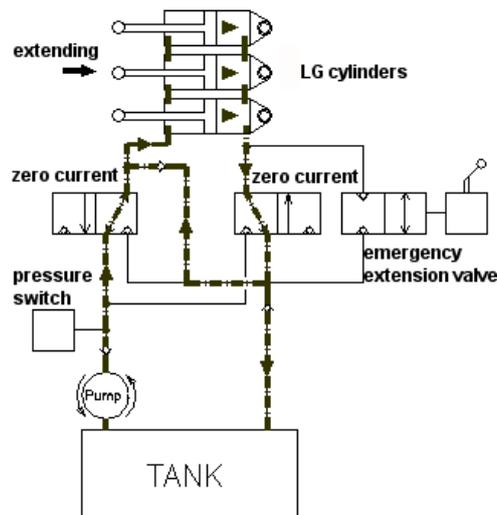
The Figure below shows the system status when the landing gear is extended. All hydraulic cylinders are under high pressure.
