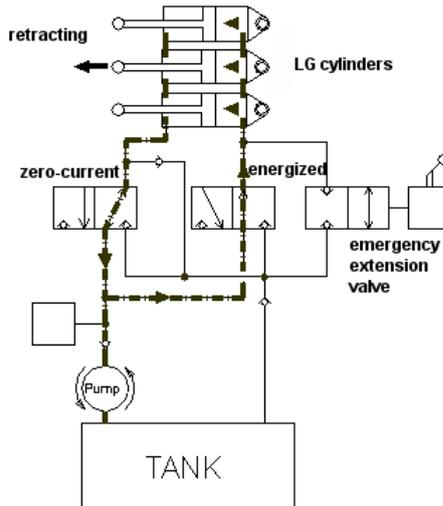
While the landing gear is retracted both valves are energized and excessive hydraulic fluid on one side is drained into the tank. This configuration of the system is shown in the following Figure.
