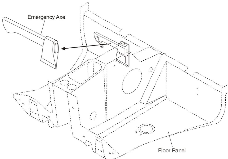
**|** Emergency Egress Hammer**|** If OÄM 42-304 is incorporated an emergency egress hammer is installed on the floor panel
