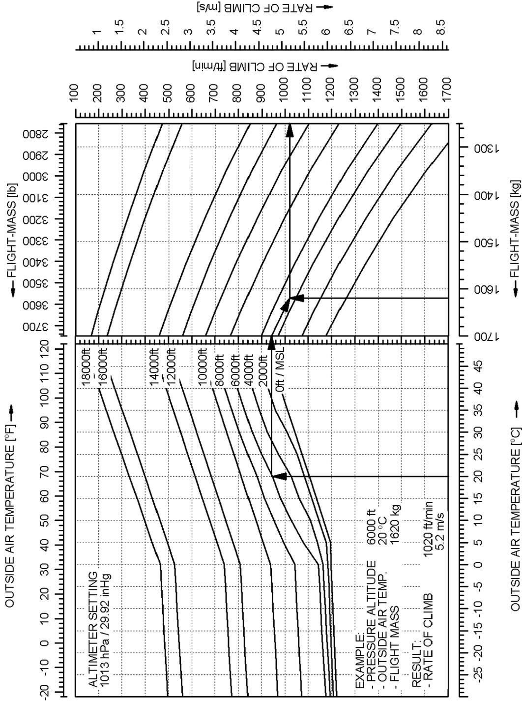
Conditions: Flaps: UP, Power: both MAX @ 2300 RPM, Landing gear: retracted, Airspeed: 77 KIAS
