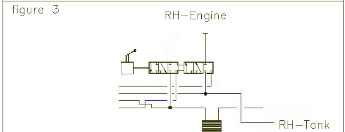
With the LH fuel selector valve in CROSSFEED position, the fuel from the RH tank is transferred to the LH engine. Depending on the position of the RH fuel selector valve, the RH tank then feeds both engines (as shown in Figure 4 below) or only the LH engine, when the fuel selector valve of the RH engine is in shut-off position (as shown in Figure 5 below).
