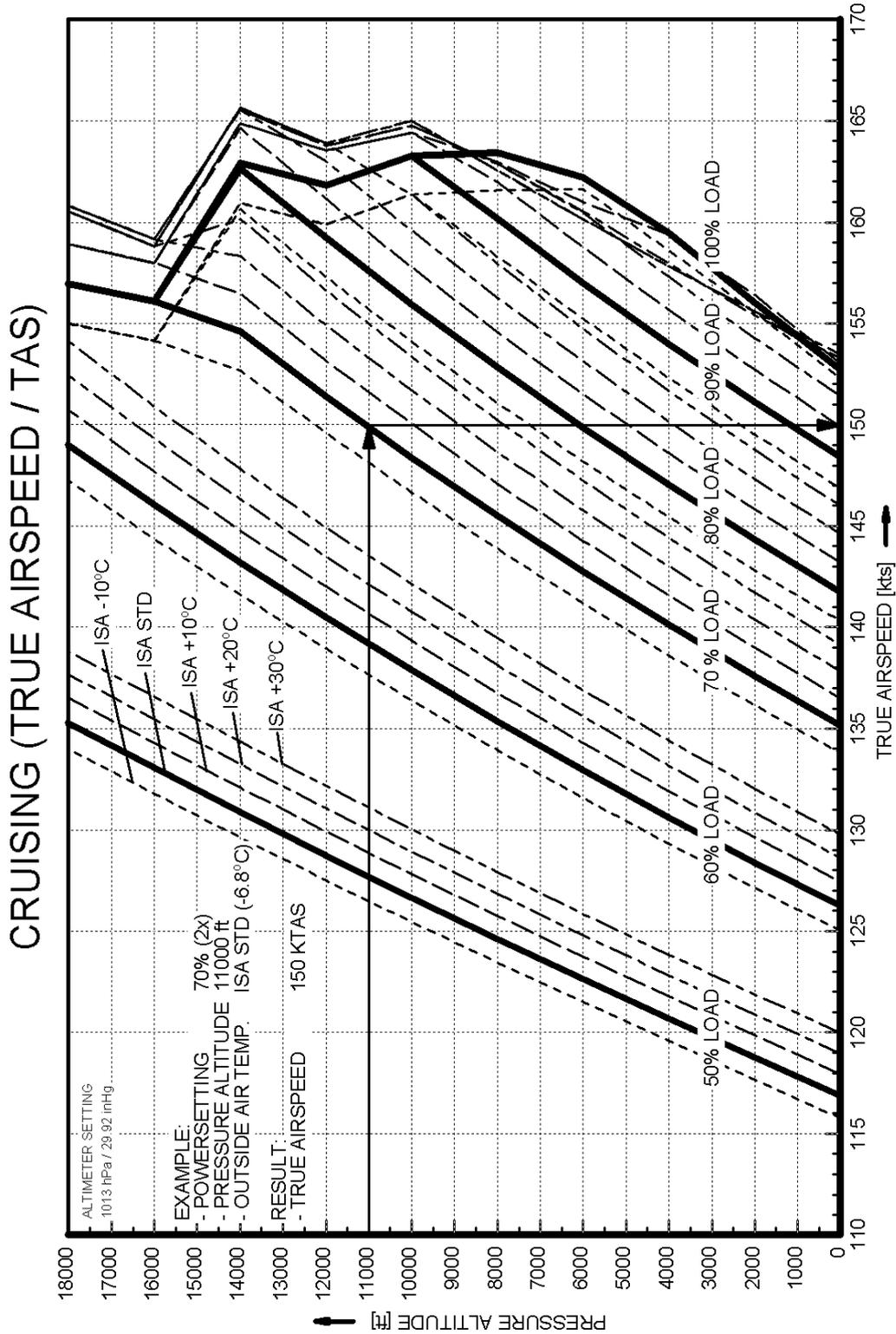
Conditions: Engines: all operating, Power: as required to adjust selected LOAD [%], Flaps: UP, Landing gear: retracted
